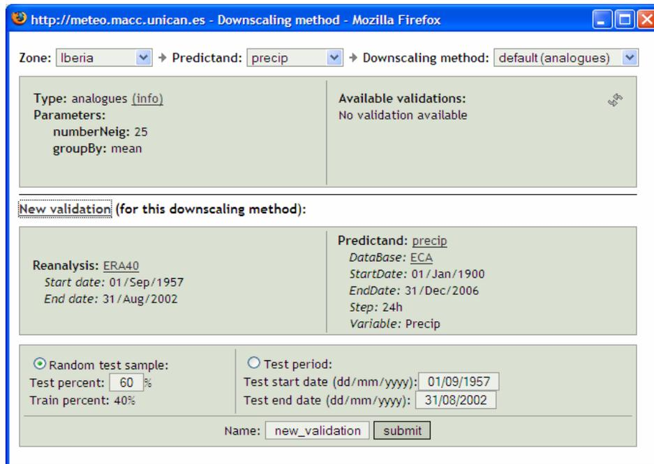
Figure 2. Downscaling methods management window. This allows the user to define and validate different downscaling methods.
